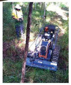
This track mounted remote-controlled flail mower can be used to create temporary fire management (control) lines. It can work on very steep slopes and being only 1.2 metres wide it can weave in between most trees. It provides a softer alternative to conventional machinery that scrapes the ground, leaving bare earth. These flail mowers are therefore especially useful to create control lines on steep slopes and erosion prone soils.
