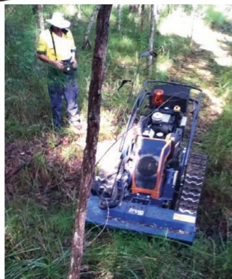
*This track mounted remote-controlled flail mower can be used to create temporary fire management (control) lines. It can work on very steep slopes and being only 1.2 metres wide it can weave in between most trees. It provides a softer alternative to conventional machinery that scrapes the ground, leaving bare earth. These flail mowers are therefore especially useful to create control lines on steep slopes and erosion prone soils.*
