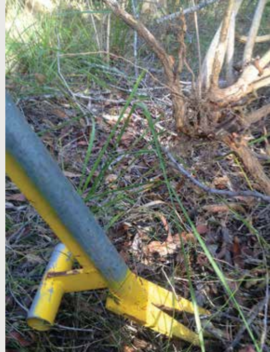
Left: Nick Clancy demonstrates the Lantana Fork, which is another useful bush regeneration tool designed to lever out woody weeds.
