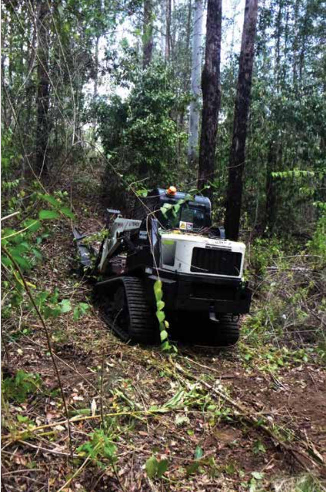
'The Terminator' - a posi-track with a front-mounted slasher was used to clear narrow, low impact, temporary containment lines.
